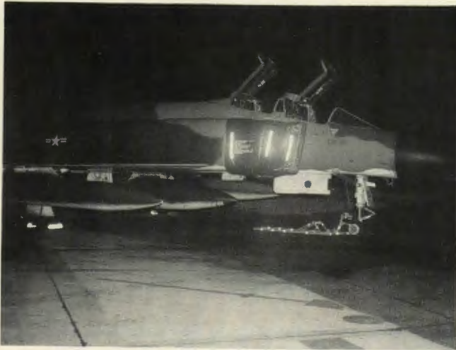
Reflective tape on ladder, chocks, intake covers, and tail hook streamer increase see-ability of camouflaged Phantom.
